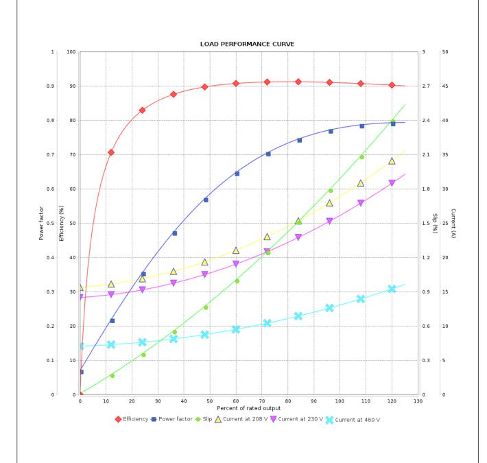
Performance : 230/460 V 60 Hz 6P Rated current : 26.5/13.3 A Moment of inertia (J) : 0.1867 kgm<sup>2</sup> **LRC** Duty cycle : 6.5 : Cont.(S1) : F Rated torque : 6.17 kgfm Insulation class Locked rotor torque : 229 % Service factor : 1.25 Breakdown torque : 280 % Temperature rise : 80 K Rated speed : 1177 rpm Design : B
