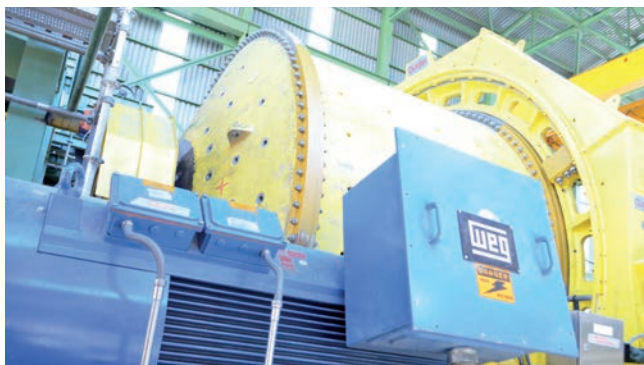
Potrerrillos Codelco Salvador - Chile Single Pinion Ball Mill - SCIM + MV VFD
