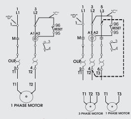
Conversion to single-phase, add jumper wire from L3 to T2 (follow dotted line connection above)
